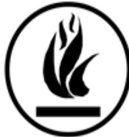
Flammable and Combustible Material
